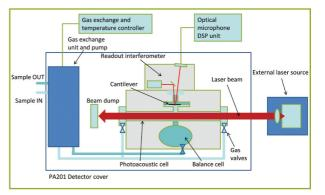
The PA201 detector includes automatic gas exchange system which can be controlled via separate controller unit.
