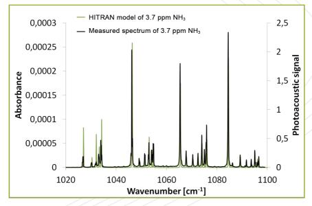
Spectrum of 3.7 ppm ammonia sample was measured using the PA201 combined with a continuous wave external cavity quantum cascade laser (CW EC QCL), which was tuned over the wavenumber range from 1020 cm<sup>-1</sup> to 1100 cm<sup>-1</sup>. Mechanical chopper was used for modulation and the maximun optical power of the laser was 62 mW.
