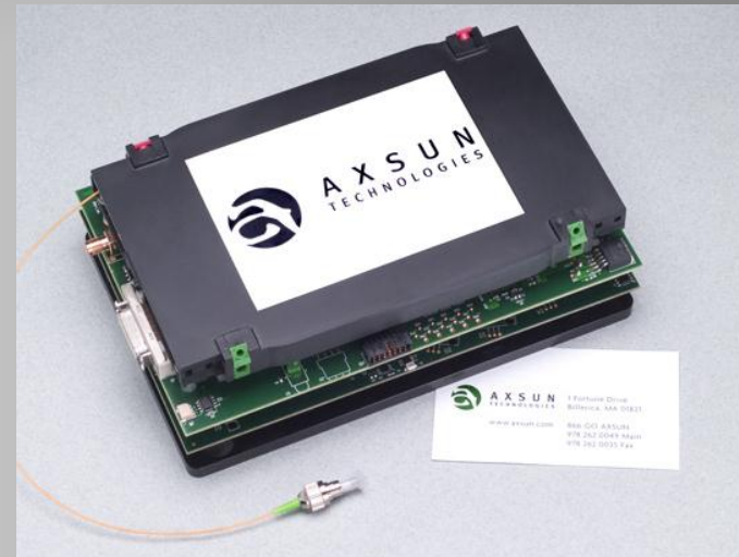
Axsun Swept Laser Engine with integrated DAQ
