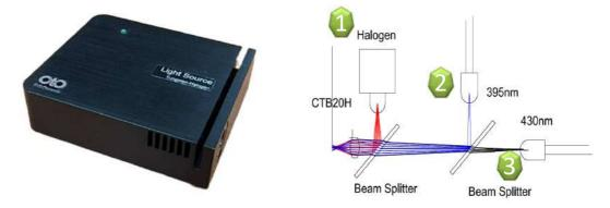
In order to align these three light spots well, the light sources are adjusted accurately. Besides the light spots are optimized, the intensity of each light source is adjusted in balance. It can provide the better measurement result. In some applications, the light source provides the flexibility to compensate the efficiency of the spectrometer.
