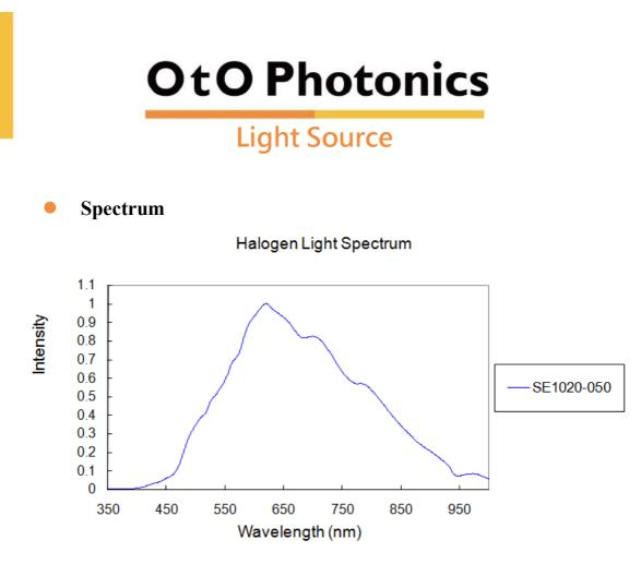
The spectrum is measured by OtO SE1020-50-VNIR (350-1020nm) spectrometer. Electrical Dark and Linearity Calibration are enabled. Intensity Calibration is disabled.
