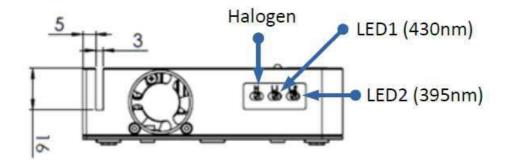
Intensity Adjustment : Halogen \ LED1(430nm) \ LED2(395nm)
