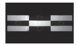
Measure values between black and white areas of the HUD projection using Checkerboard Contrast to test contrast.
