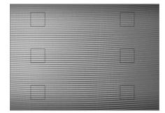
Use Modulation Transfer Function (MTF) line pair algorithms to calculate contrast at different spatial frequencies to determine image clarity. Testing uses horizontal and vertical pairs of black and white lines.
