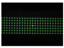
Test distortion of the virtual image using Distortion Dot Grid to measure the spatial offset between dots of the primary image and a test pattern. Distortion can also be tested using Distortion Line Grid Analysis.
