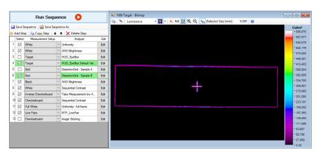
Apply tests separately or in sequence to evaluate all critical display quality parameters. TT-HUD can integrate with the HUD system to control display test images in conjunction with the test sequence for production-level automation.
