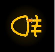
**Inspection and defect detection:** Evaluate the integrity of icons and shapes against trained templates. Ensure regions are free from defects, such as unintended inclusions or exclusions, caused by inaccurate laser etch or errors in overlays, filters, and other substrate layers.
